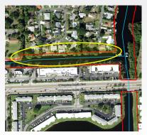
E-1E - Little to no usable ROW on either bank, extensive docks, embankments and encroachments; some sections are wide and deep, and adjoining property is steeply graded
